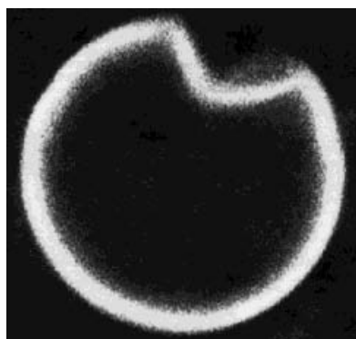
Figure 2. A confocal micrograph of an 8- \mu\text{m} hollow sphere illustrating the stability and deformability of a [(PSS/PAH) 4 PSS] hollow shell. [3]
